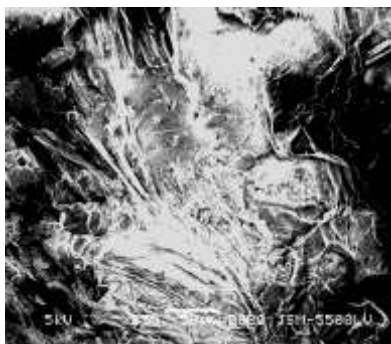
Fig. ( 36 ) crystallization of Halite and Gypsum which caused disintegration of the lime mortan
