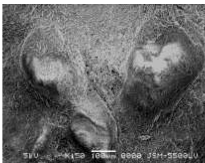
Fig. ( 37 ) Quartz as filler material in the lime mortar embedded in Calcite as binding material after carbonation process of the slacked lime
