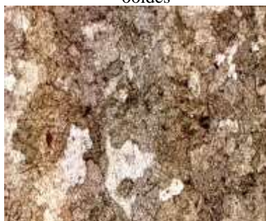
Fig.( 29 ) P.M. view of white Calcite ( two sets of cleavages ,Dolomite ,and Quartz
