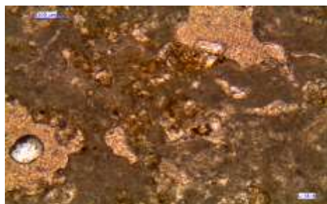
Fig. ( 44 ) Stereomicroscope view shown of marble sample Calcite and erosion of surface .
