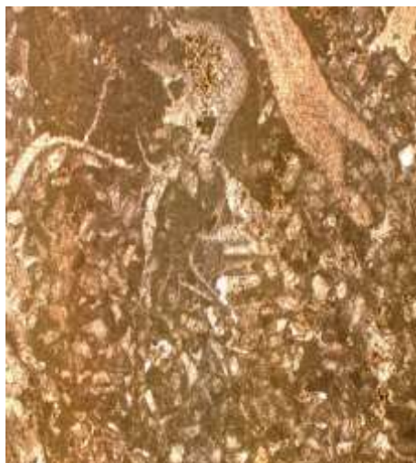
Fig.( 31 ) P.M. view of gray marble remains, vermetids ,Gastropod shells, Lithophyllum , foraminifera
