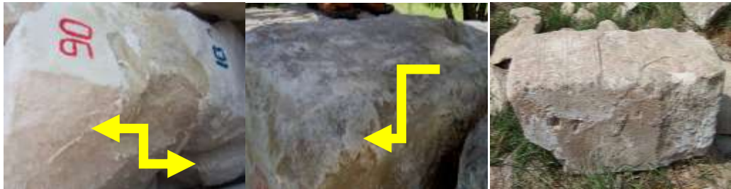
Fig. (3a,b) crystallization of different salts to light-colored crust tracing the surface and between layers of engraved limestone.
