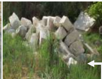
Fig. (16) Wrong storage between grass and areas of high humidity
