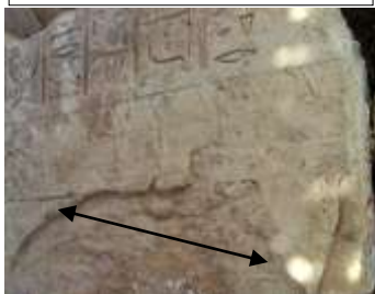
Fig. 9 shows the disintegration of the engraving limestone.
